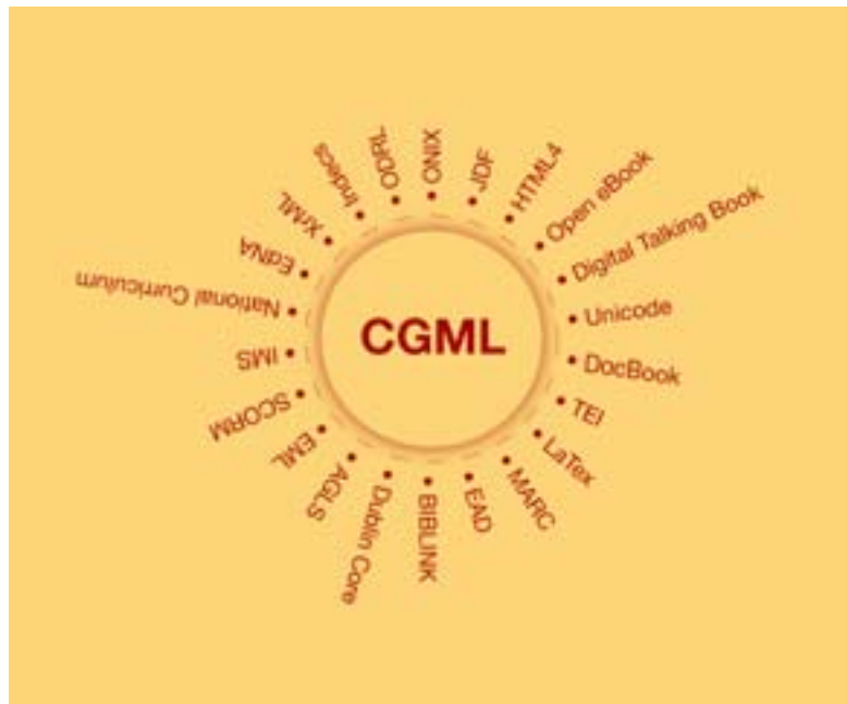
Figure 3. The interlanguage approach – full interoperability between 17 schemas requires a thesaurus with just 17 sets of tag synonyms.
